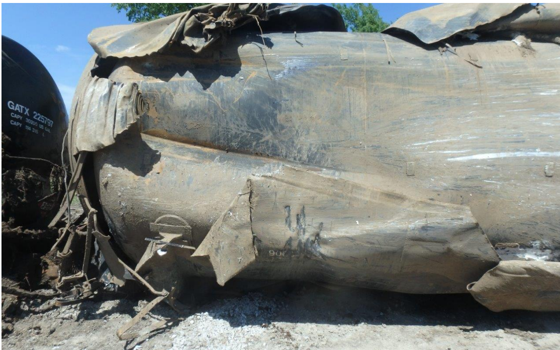
Figure 2. DOT-117J100W tank car, which sustained impact damage, but did not release denatured ethanol.
