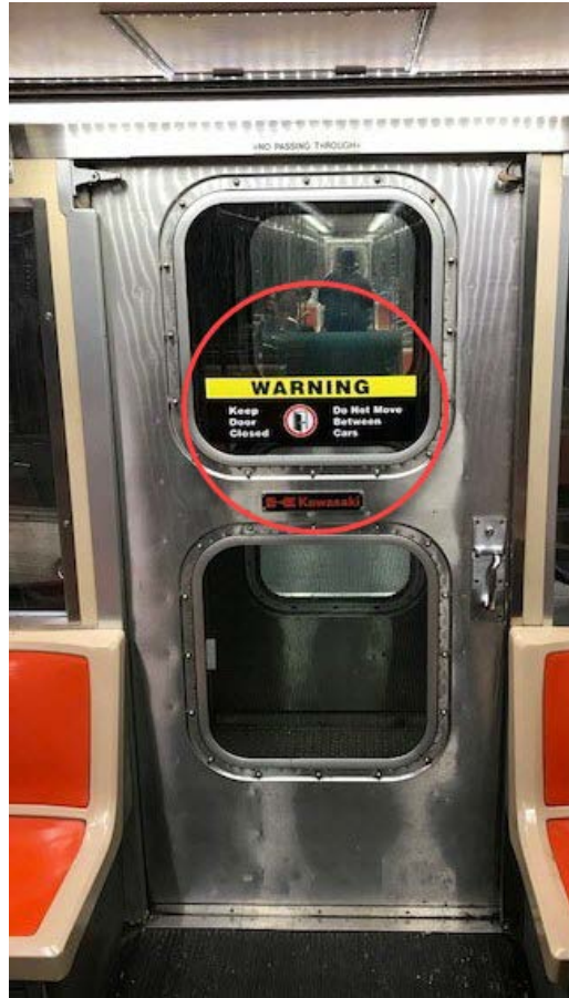
Figure 3. Photograph of an enhanced warning sign on a SEPTA subway end-of-car door.
