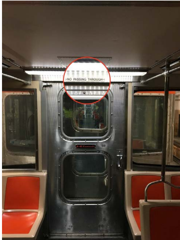
Figure 2. Photograph of a SEPTA subway end-of-car door warning sign.
