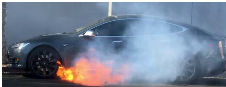
Figure 2. View of the left side of the Tesla, showing flames coming from the vehicle's underside. (Source: bystander video)
