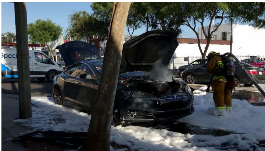
Figure 3. View of the Tesla and a firefighter after water and foam had been applied to the vehicle. (Source: Tesla Inc.)
