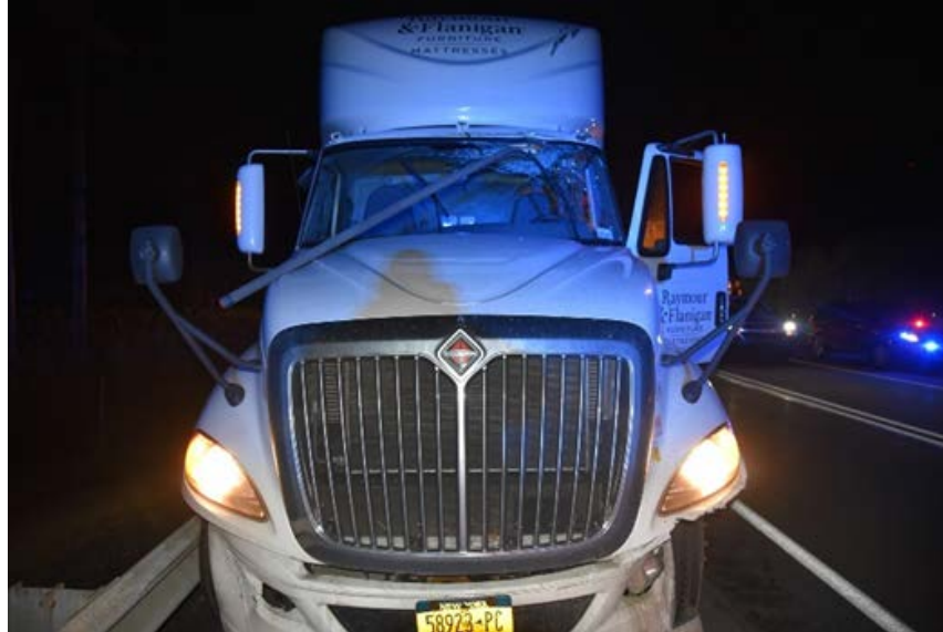
Figure 2. Front view of the combination vehicle at its final rest position. The displaced section of electrical conduit can be seen resting on the corner of the hood, with the end protruding through the upper part of the windshield. (Source: Pennsylvania State Police)
