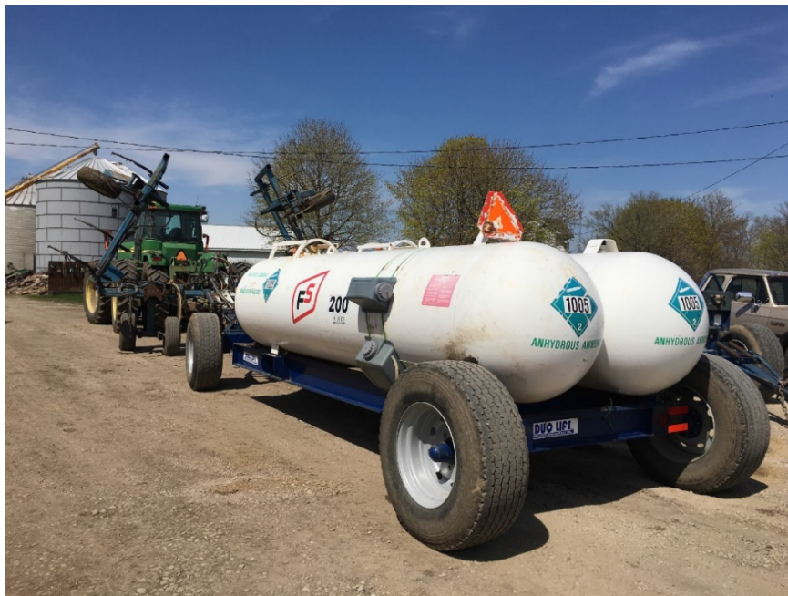
Figure 1: Photo of John Deere tractor with the applicator tool and nurse tanks attached.
