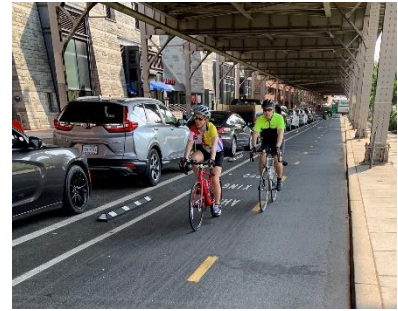
c. Two-way separated bike lane with parking as barrier
