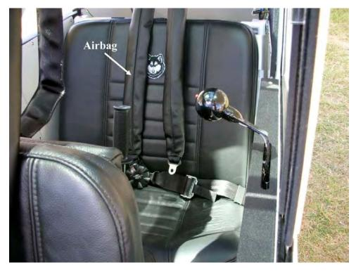
**Figure 19.** A photograph of exemplar Aviat Husky airplane seats with airbags mounted in the right shoulder harness.<sup>85</sup>
