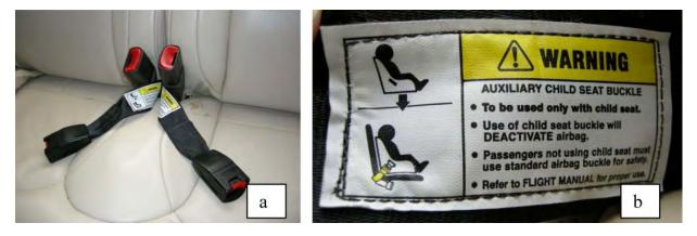
**Figure 43.** A pair of photographs showing seat belt buckles and a buckle label. Photograph a, on the left, shows the primary (top) and child seat (bottom) buckles for the rear seat occupants. Photograph b, on the right, shows the label stitched to the child seat buckles.
