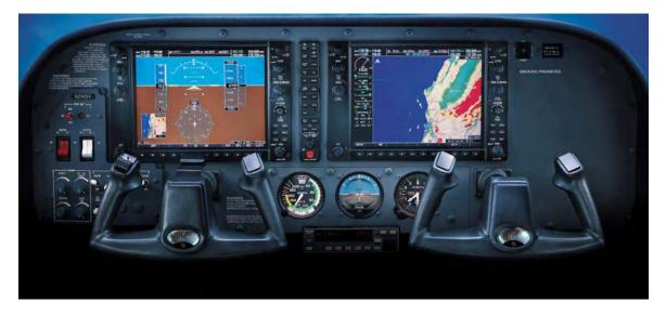
**Figure 14.** A photograph of the Cessna 172 Skyhawk instrument panel.<sup>81</sup> The Skylane panel has a similar glass cockpit panel with dual control yokes.
