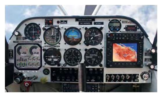
**Figure 18.** A photograph of the exemplar Aviat Husky A-1B instrument panel. (Radio Package 2 panel shown.)<sup>84</sup>
