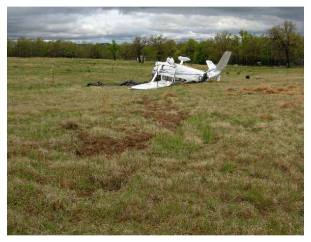
**Figure 42.** A photograph showing the final resting position of Cessna 182T, N1491D, which crashed in Stigler, Oklahoma. Two major impacts of the nose into the ground are visible in the foreground.
