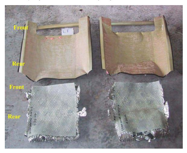
**Figure 26.** A photograph showing the seat pan and aluminum EAMs from the two front seats. The left front seat pan and EAM block are on the left side of the photograph. The front of both seat pans is toward the top of the photograph.
