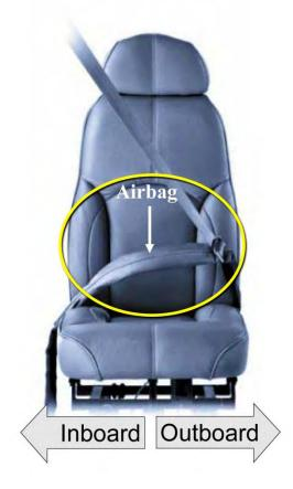
Figure 15. A photograph of an exemplar Cessna airplane seat with a lap belt-mounted airbag system.  $^{\rm 82}$
