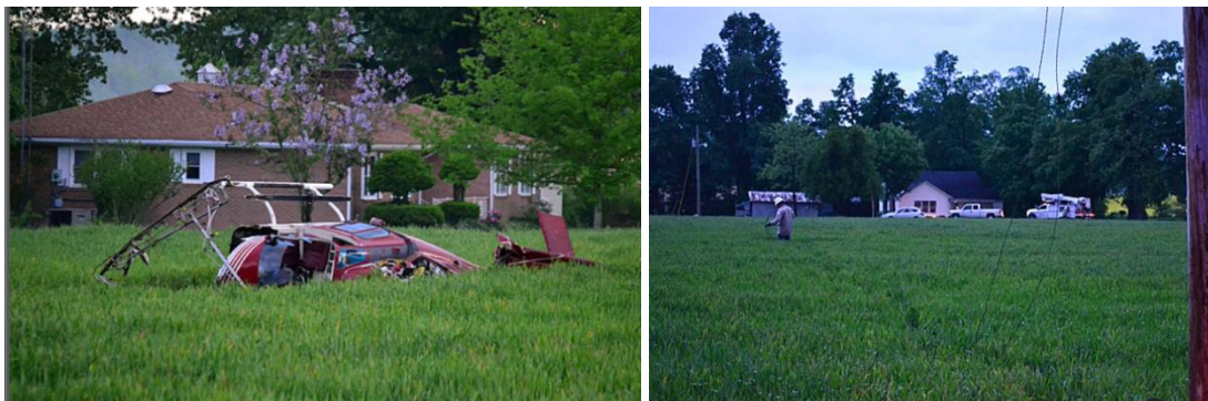
Figure 5. Wreckage of a Bell 206B that struck power lines (left) and the severed lines (right).
