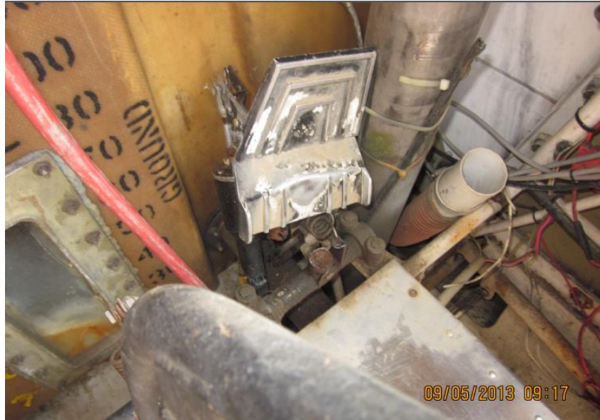
Figure 6. Damaged rudder pedal of a Cessna 188B airplane.
