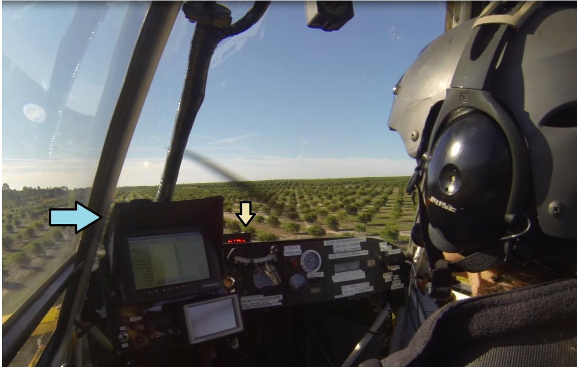
Figure 4. GPS swath guidance system installed in a two-seat training aircraft.
