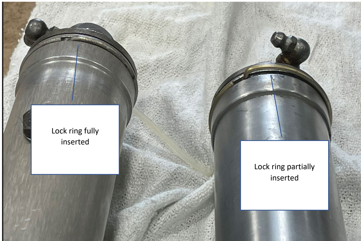
Figure 8. Exemplar horizontal stabilizer actuators and lock rings.
