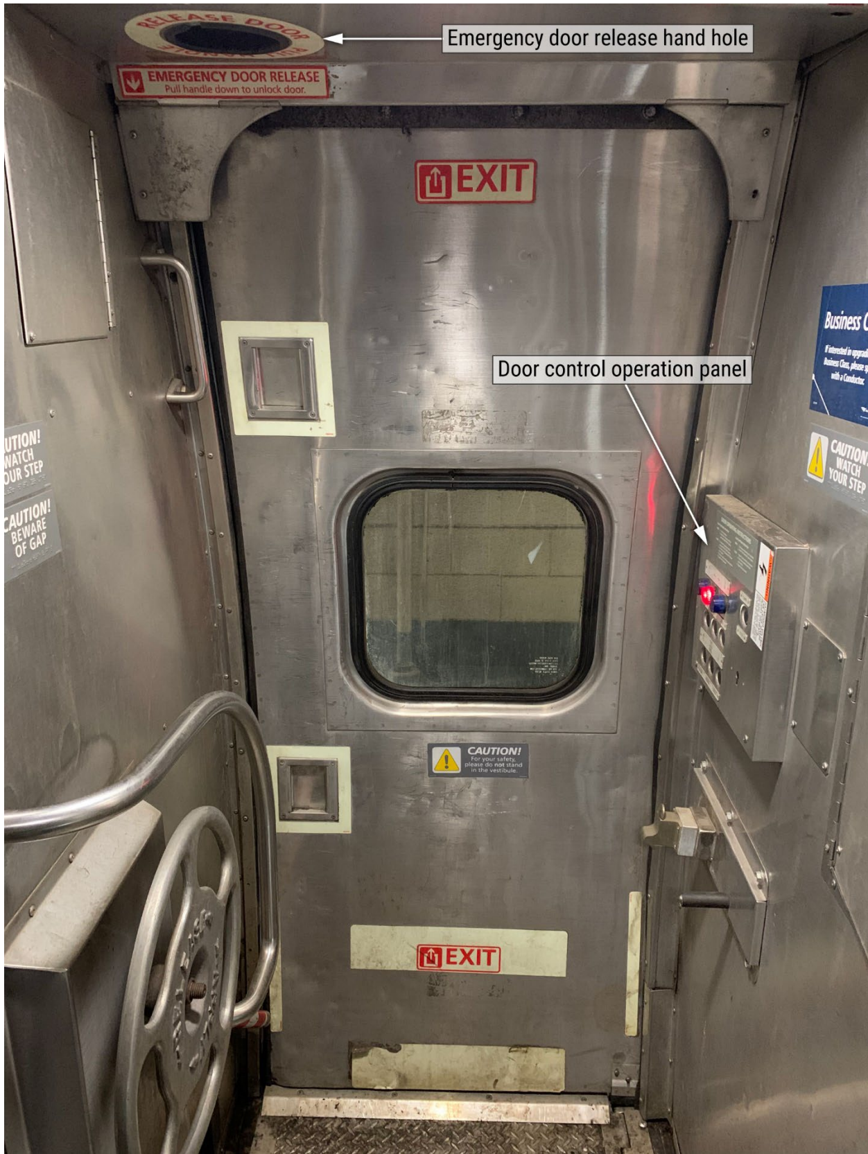
Figure 2. Example of an Amfleet 1 exterior side door. (Photograph courtesy of Amtrak.)
