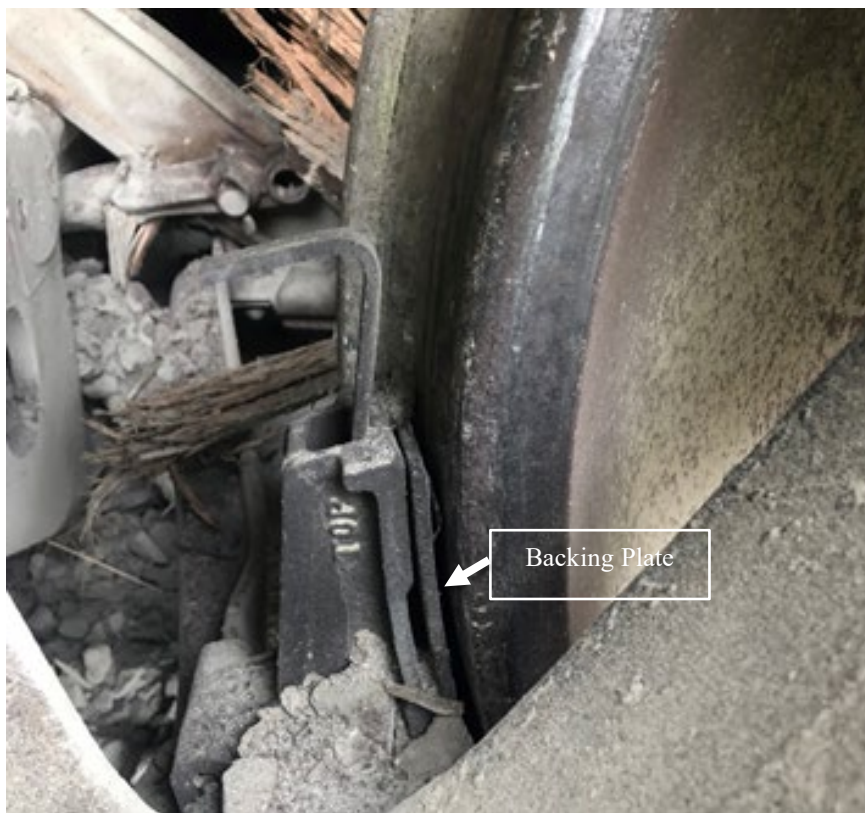
Figure 4. Striking train's wheel set. Composite material is worn off the brake shoe.
