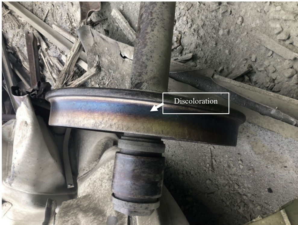
Figure 3. Wheel set from the striking train. The blue discoloration indicates overheating.
