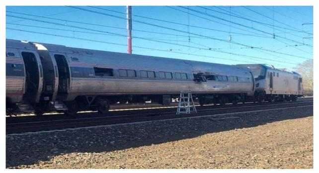
Figure 9. Damage to lead passenger car.
