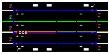
**Figure 6.** Dispatcher's display screen at 7:34 a.m. with a clear signal for train movement on track 3 indicated by the green highlight.
