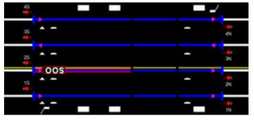
**Figure 4.** Dispatcher's display screen at 7:25 a.m. showing tracks 1–4 between Control Points Baldwin and Hook. Track 2 is out of service track (magenta), and tracks 1, 3, and 4 have electronic blocks (blue).
