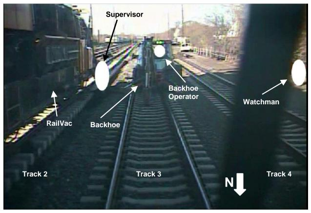
Figure 3. RailVac and backhoe taken from forward-facing video recorder just before accident.
