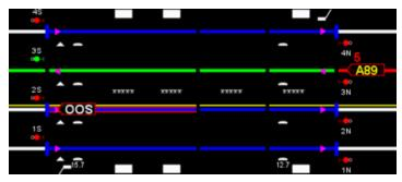
Figure 7. Dispatcher's display screen at 7:47 a.m. with train 89 on track 3 shown by the A89 designation.
