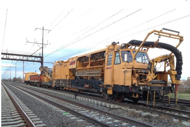
Figure 2. RailVac vacuum excavation machine on track 2 at the accident site.
