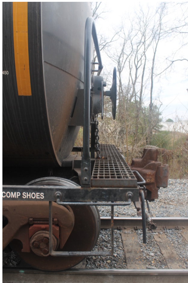
Figure 2. Photo of end platform on an exemplar tank car that the RCL operator was riding. (Source: FRA)
