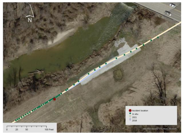
**Figure 3.** IMU data for Woodpat pipeline from 2018 and 2021 and 2022 postaccident GPS survey.
