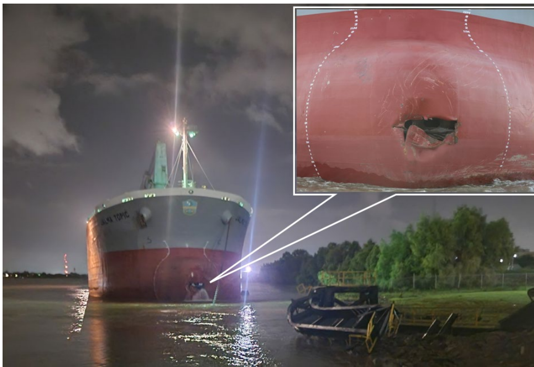
Figure 5. Jalma Topic down river of the office barge at 0328 with its port anchor out. Inset shows a close-up of the damage to the vessel's bulbous bow. (Background source: J. Claverie)
