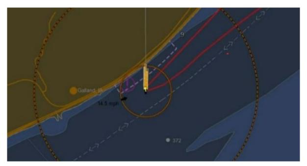
**Figure 3.** Snapshot of *Baxter Southern* ECS playback at 2336 showing the area marked by a magenta dashed line and the vessel pushed up against the riverbank. (Source: Southern Towing Company)
