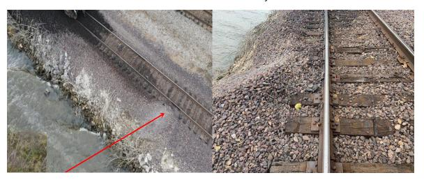
**Figure 8**. Aerial drone photo of the casualty site with a red arrow pointing to the indentation remaining in the ground where the forwardmost barge *STC 3020* was located (*left*). Close-up of the indentation from the barge in the shoreline next to the railroad track (*right*). (Sources: BNSF [*left*], Coast Guard [*right*])
