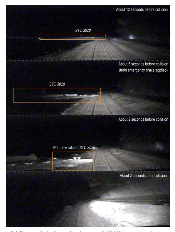
**Figure 5**. Still images of video footage from locomotive BNSF 9251's recorder as the train approached the barge and derailed after hitting the barge. The forward barge of the *Baxter Southern* tow is outlined in orange. (Source: BNSF)
