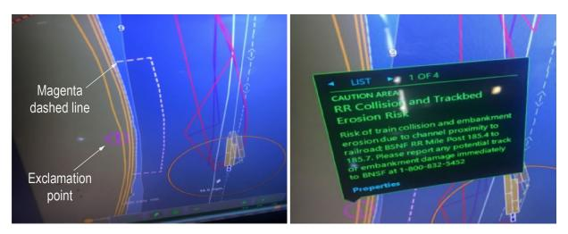
**Figure 9.** Baxter Southern Rose Point in nighttime display showing the area marked by the magenta dashed line and exclamation point (*left, annotated by NTSB*) and information contained in the corresponding caution note (*right*). (Source: Southern Towing Company)
