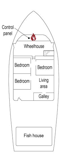
**Figure 3.** Main deck general layout (not to scale) with location of fire indicated by flame symbol.
