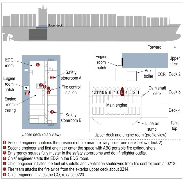
**Figure 3.** Profile view of the *President Eisenhower* (*top*). Plan view of the upper deck showing the sequence of events during the fire (*left*). Profile of the upper deck and engine room decks with the origin of fire highlighted (*right*).
