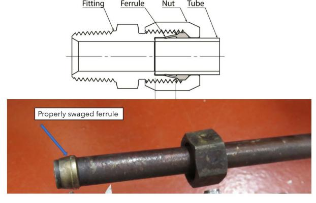
**Figure 5.** Cross-sectional diagram of typical compression fitting and body (*top*). Properly swaged ferrule on the *President Eisenhower*'s old section of fuel oil return tubing (*bottom*). (Top source: Worldwide Fittings)
