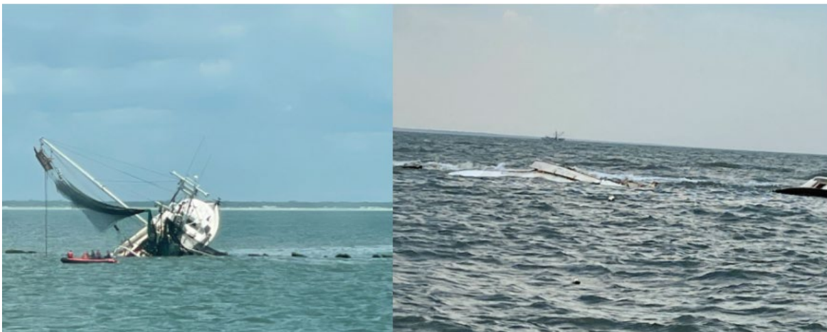
Figure 5. Sage Catherine Lane following the grounding on the jetty (left), and after being broken apart on the jetty 3 days later (right). (Source: Coast Guard)
