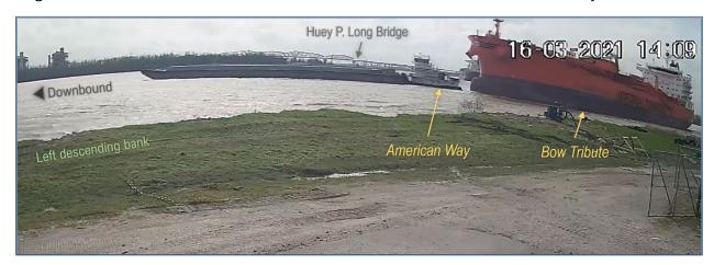
**Figure 4.** CCTV footage looking upriver at 1521 shows the *Bow Tribute* near the left descending bank with the *American Way* by the tanker's starboard bow. (Timestamp is 1 hour 11 minutes behind the actual time.) (Source: Crosby Dredging)
