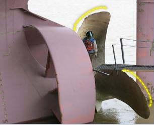
**Figure 6.** Postcasualty damage to the *Bow Tribute's* portside aft hull (*left*) and propeller (*right*), as indicated by yellow dashed lines.
