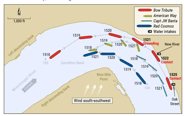
**Figure 3.** Positions of the *Bow Tribute*, *American Way*, *Capt JW Banta*, and *Red Cosmos* (approximate scale) in the Carrollton Bend in the minutes leading up to the casualty, based on automatic identification system data. The *Bow Tribute's* subsequent contact at the two river intakes is also identified.
