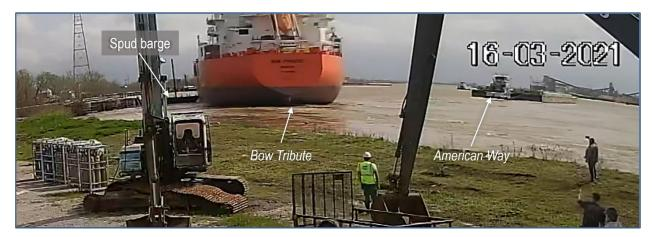
**Figure 5.** CCTV footage looking downriver at 1522:26 shows the *Bow Tribute* when it struck the spud barge protecting the New River water intake pipes. (Source: Crosby Dredging)
