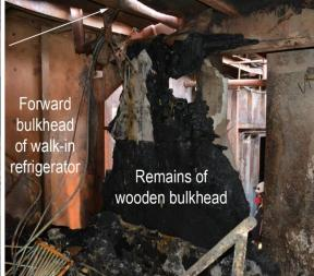
**Figure 8.** Forward end of *Aleutian Falcon* walk-in refrigerator after the fire. (Background source: ATF)
