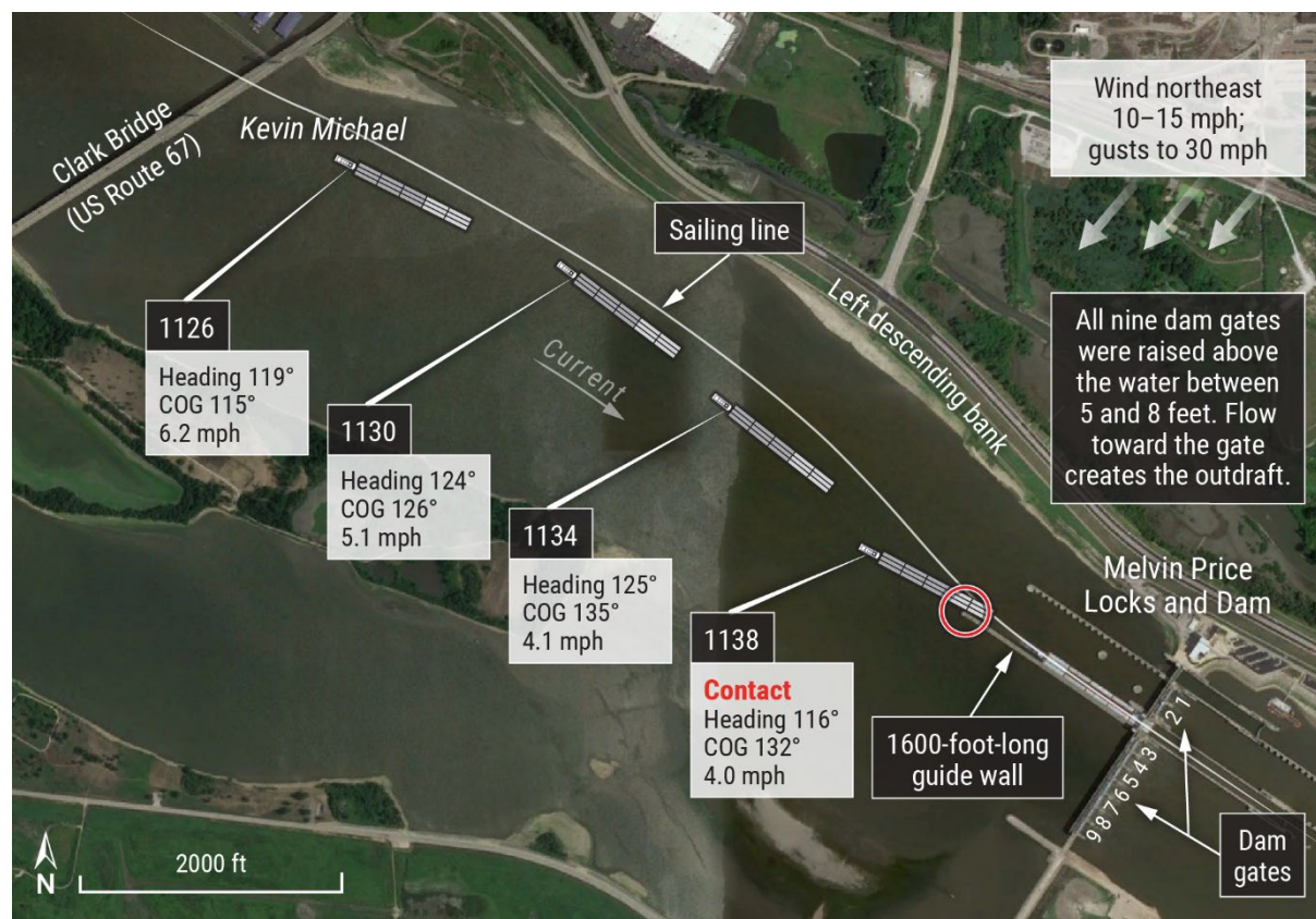
Figure 4. Annotated electronic chart system track history of the Kevin Michael tow over the last 12 minutes leading up to the casualty. (Background source: Google Earth)
