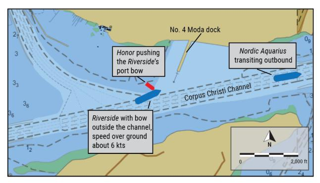
**Figure 4.** Approximation of *Riverside* at 1300, just before the contact with the no. 4 Moda dock dolphin and catwalk, with the tug *Honor* pushing its port bow; the *Nordic Aquarius* has departed the no. 4 Moda dock and is transiting outbound. (Background source: NOAA)
