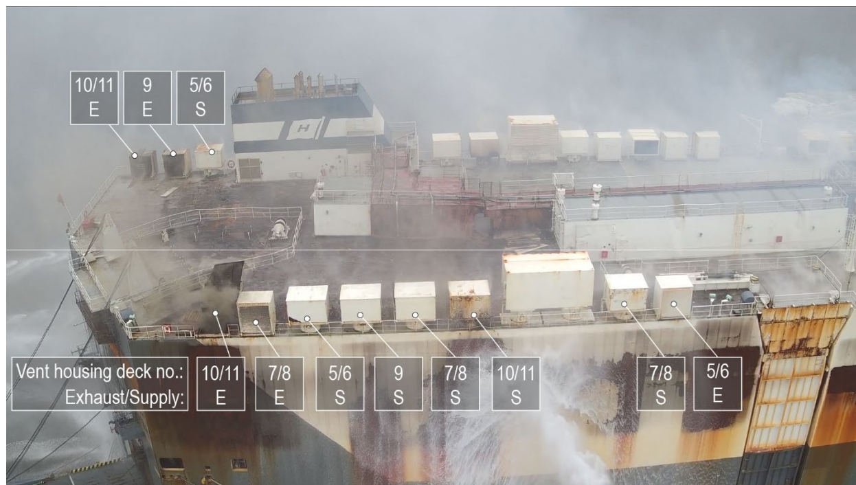
Figure 11. Damaged aft ventilation housings after the reported explosion of portside vent housing for deck 9 (9E in the photo). (Background source: JFRD)
