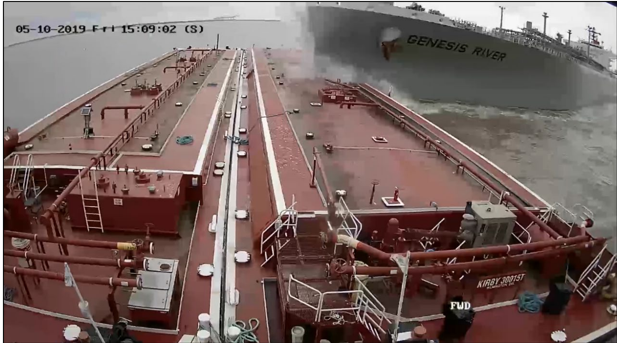
Figure 8. Screen capture from wheelhouse video on board the Voyager at the moment that the Genesis River struck barge 30015T. (Source: Kirby Inland Marine, LP)
