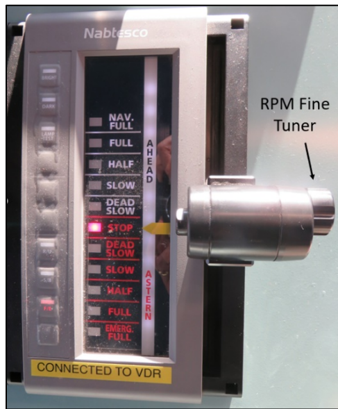
Figure 9. Genesis River bridge EOT lever.
