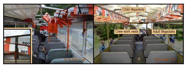
**Figure 13.** Lifejackets recovered on the *Stretch Duck 7* (*left*) compared to how they would have been stowed, as shown on the similar vessel *Stretch Duck 9* (*right*). Infant lifejackets would have been stowed aft of the child lifejackets. (Source: Missouri State Highway Patrol)
