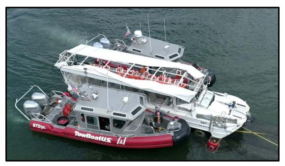
Figure 11. Torn canopy on the Stretch Duck 7 during recovery at Table Rock Lake.
