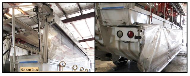
**Figure 12.** Closed starboard-side curtain as found during recovery (*left*) and then released (*right*) during the postaccident investigation.
