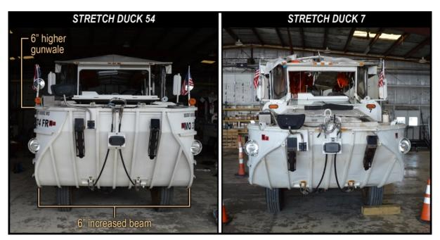
**Figure 9.** As shown in these photos taken postaccident, the *Stretch Duck 54*, a later model of the stretch duck known as a master jig, had a larger beam and higher gunwale than the *Stretch Duck 7*.
