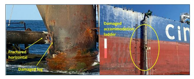
Figure 5. Damage to SP-57B (left) and Atina (right). (Source: Coast Guard)
