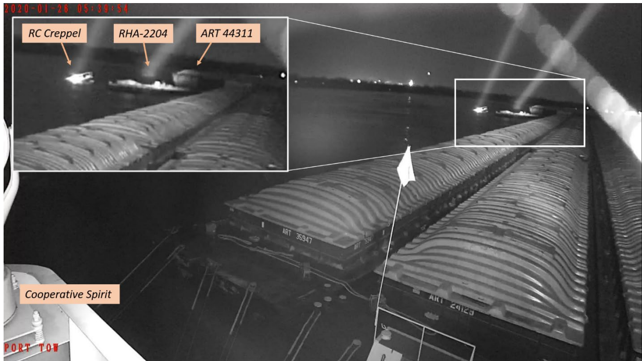
Cooperative Spirit port camera screenshot of the mostly submerged RC Creppel and barge ART 44311 on top of barge RHA-2204 at 0539:54. (Source: ARTCO, annotated by NTSB)
