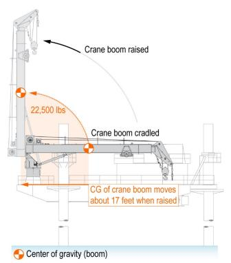
When the captain raised the *Kristin Faye*'s port crane boom, its center of gravity shifted about 17 feet.
