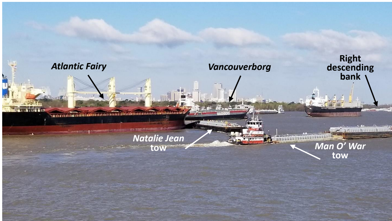
Photo (looking upriver) of the Natalie Jean tow perpendicular to the Atlantic Fairy . The towboat has capsized and is sinking. (Photo by Moran Towing)
