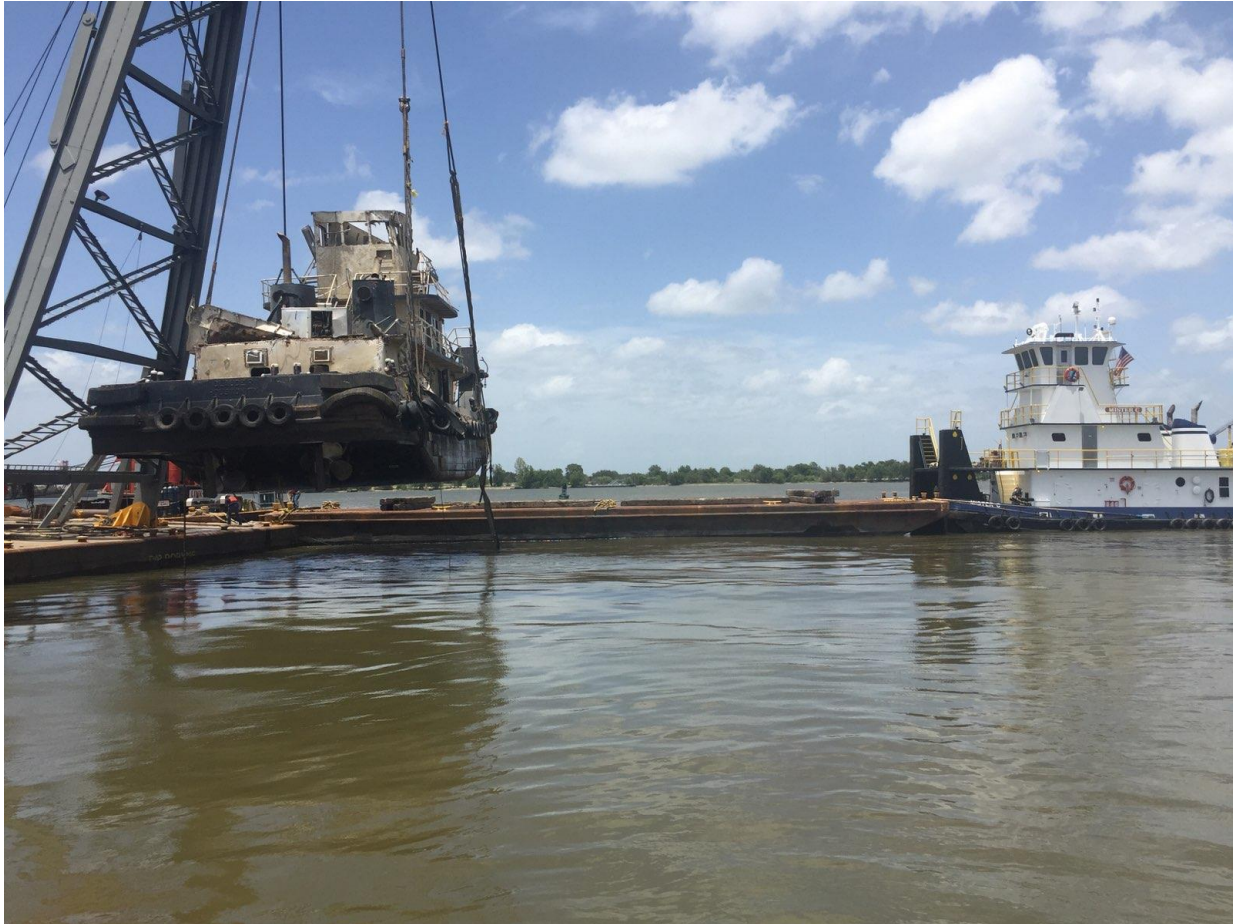
Natalie Jean being salvaged. The vessel was upside down on the river bottom and sustained damage to the shaft and flanking rudders in the recovery efforts. (Photo by Coast Guard)
