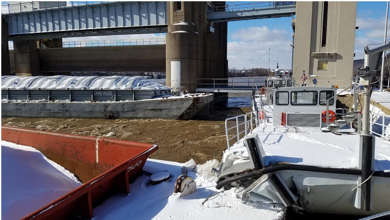
Stern of barge C508 after colliding with Corps of Engineers workboats Emsworth (foreground) and Dashields (background). (Photo by Coast Guard)
