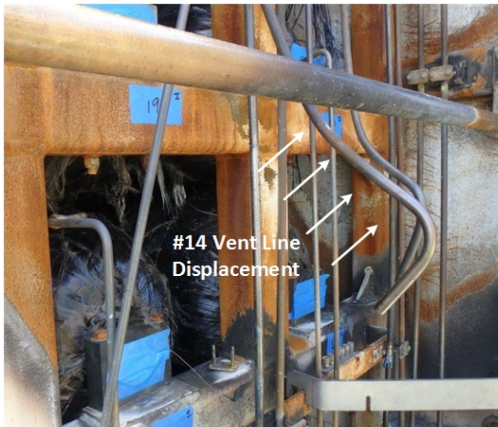
Figure 9. No. 14 vent line displacement. The vent line was bent outward from the cylinder and against the handhold rail. March 12, 2018.
