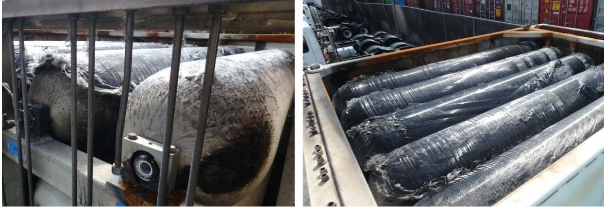
Figure 7. Cylinders 21 through 25 thermal damage with protective fiberglass and epoxy coating burned away, March 14, 2018.
