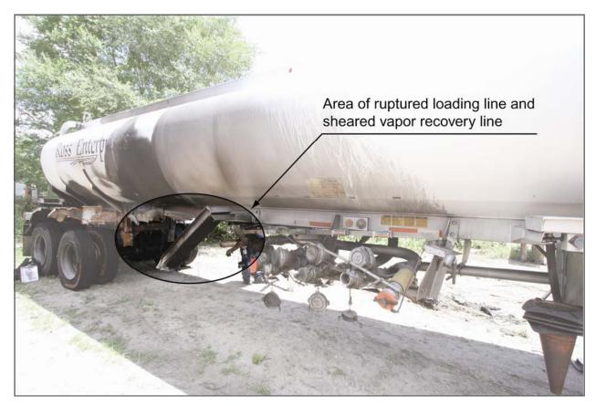
Figure 2. Rear passenger side of accident cargo tank truck showing external damage from collision and fire.
