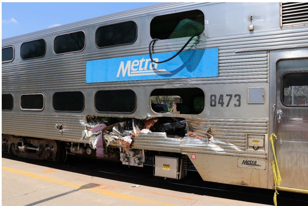
Figure 5. Exterior damage to the lower-level seating area of the right side of the commuter train's lead cab car. The upper level also sustained window damage.
