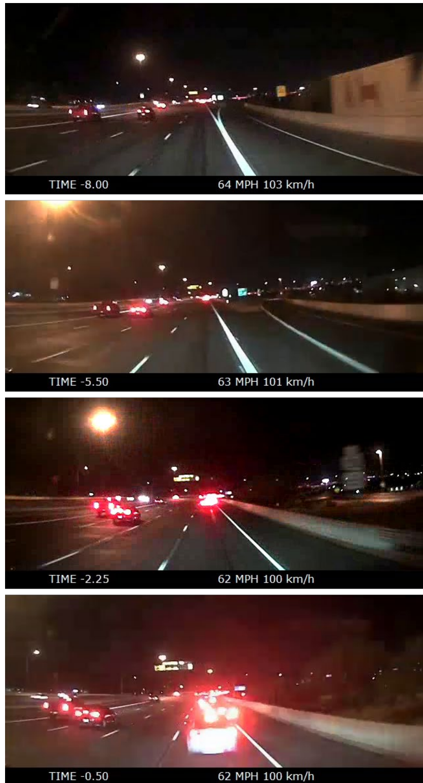
Figure 8. Capture of the video from truck-tractor's forward-facing camera at 8 seconds (top image), 5.5 seconds (second image from top), 2.2 seconds (third image), and 0.5 seconds (fourth image) before impact.
