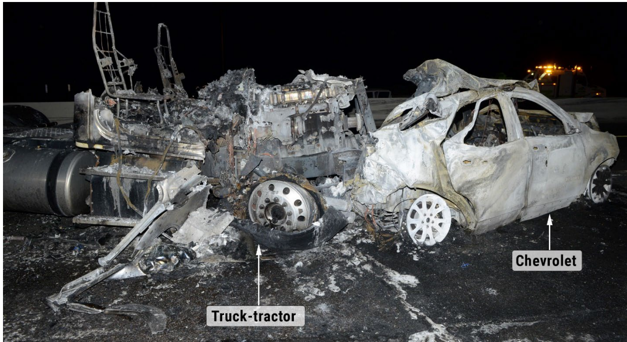
Figure 3. At-rest positions of the truck-tractor and Chevrolet. (Source: AZDPS with annotations by the NTSB)
