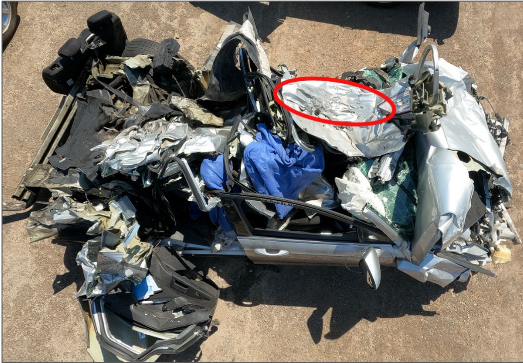
Figure 9. Overhead view of damage to Ford. The red circle on the vehicle's roof highlights tire marks made by the truck-tractor.
