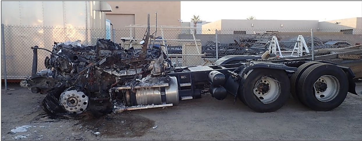
Figure 6. View of damage to the left side of truck-tractor.
