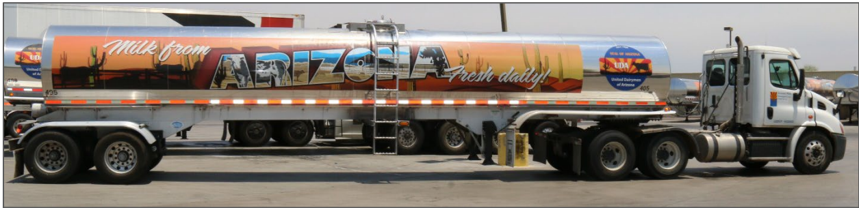
Figure 5. Right-side view of an exemplar combination vehicle with AMT truck-tractor and UDA tank-trailer.
