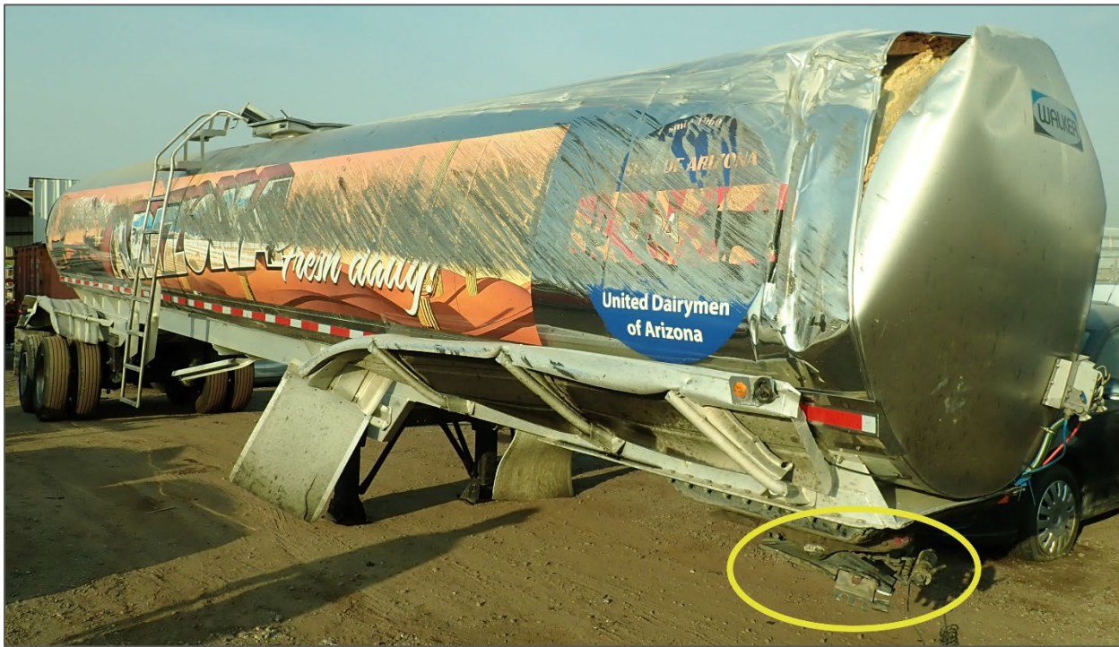
Figure 7. View of damage to the front and right side of tank-trailer. The yellow circle highlights the fifth wheel assembly.
