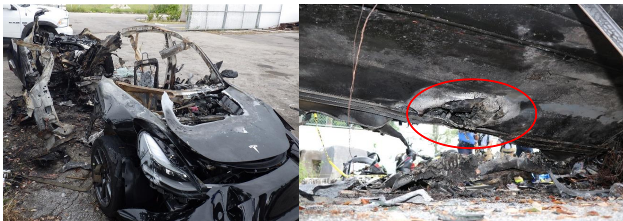
Figure 6. Impact damage to passenger side and fire damage to car (left), with burn hole in battery case circled in red (right).
