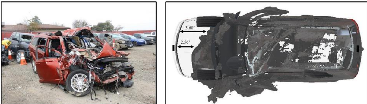
Figure 4. Left image depicts damage to front and right side of SUV. Right image is overhead view of 3D laser scan of SUV overlaid on exemplar vehicle.
