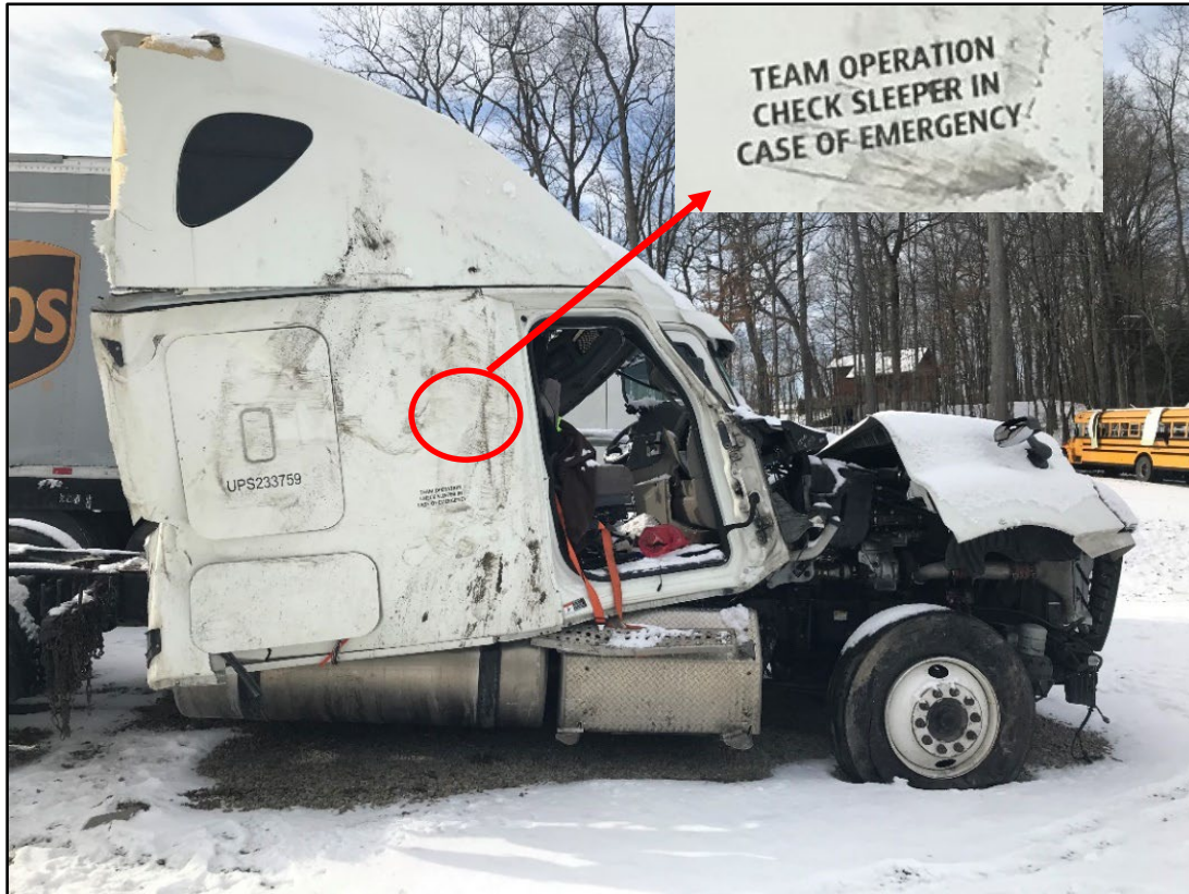
Figure 5. Right side of UPS-1 showing sign telling emergency responders to check truck's sleeper berth.
