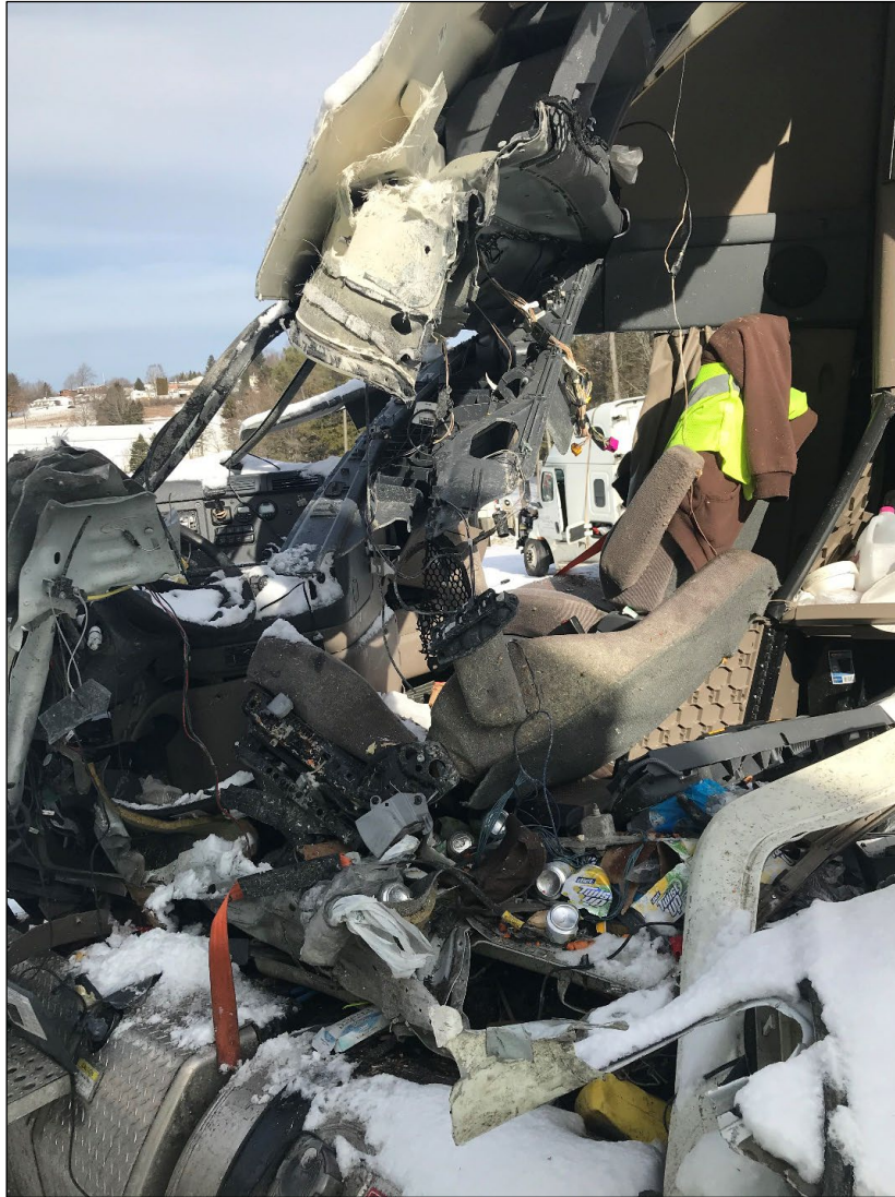
Figure 13. Damage to interior of UPS-1 cab, showing position of driver's seat and destruction to controls.
