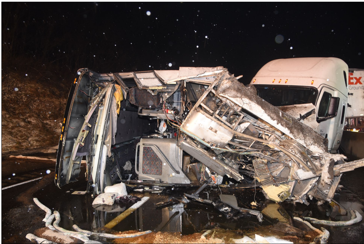
Figure 7. Photograph of collision scene showing front of motorcoach rolled onto its right side and entangled with front of FedEx truck. (Source: Pennsylvania State Police)
