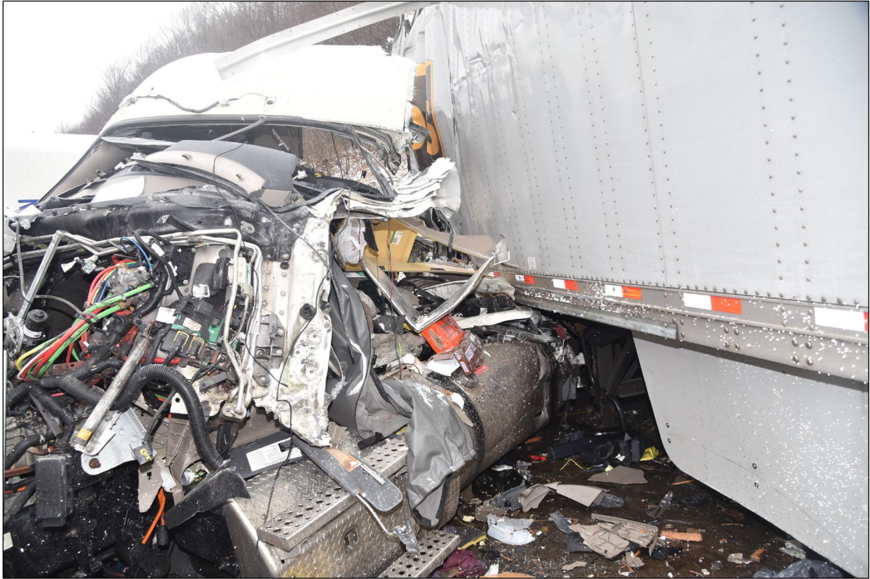
Figure 12. Photograph taken at scene showing damage to UPS-1 cab.(Source: Pennsylvania State Police)
