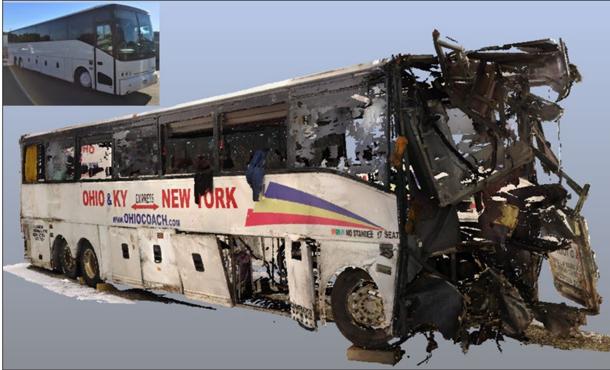
Figure 8. Point-cloud image of motorcoach postcrash, with inset photo of intact motorcoach of same model.
