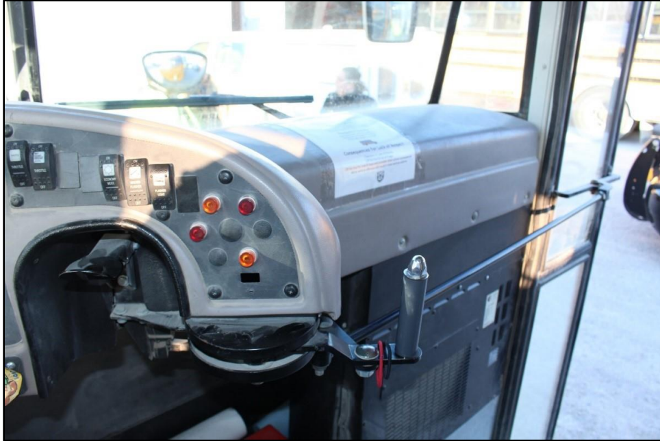
Figure 13. Manually operated loading door at front of exemplar bus, showing hand-operated lever and connecting rod to door.
