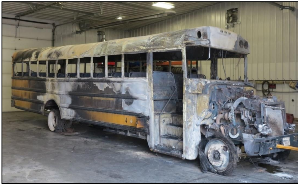
Figure 6. Fire damage to bus's front and right side, including loading door, windows, roof, and engine (photographed after bus was removed to garage).
