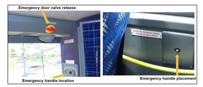
Figure 6. Interior of the motorcoach, showing the three assemblies necessary to open the rear door.
