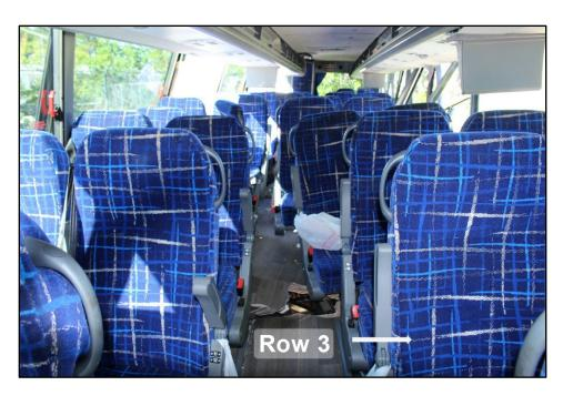
Figure 5. Motorcoach interior, showing the buckling of the floor and the lateral displacement of the seats.
