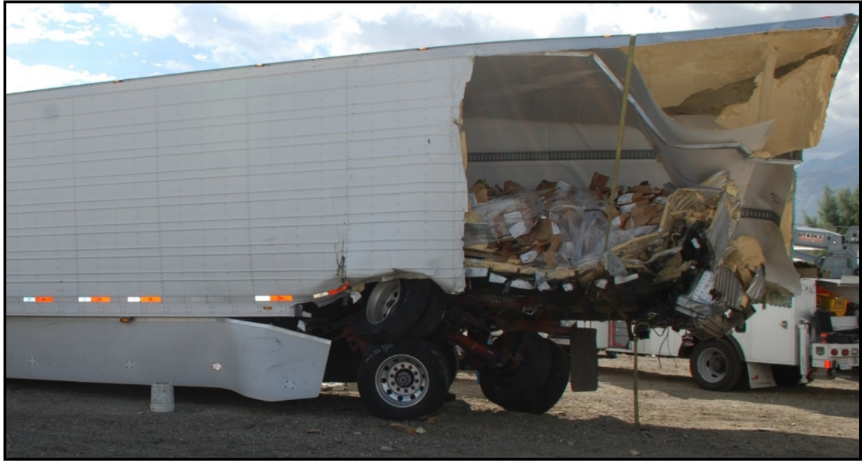
Figure 7. Semitrailer postcrash, showing extensive rear damage. (Source: California Highway Patrol)
