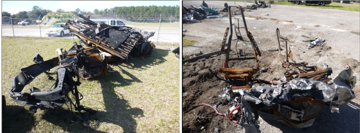
Figure 5. Damage to the Eagle Express truck-tractor (left) and its driver and passenger seats (right).
