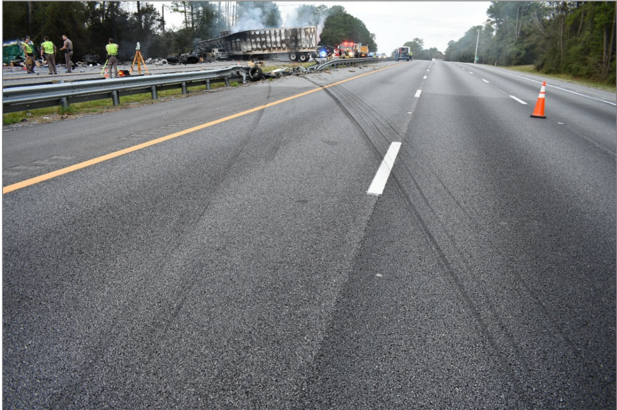
Figure 2. Northbound view of the crash scene, including tire marks from the leftward arc of the Eagle Express truck. (Source: Florida Highway Patrol)
