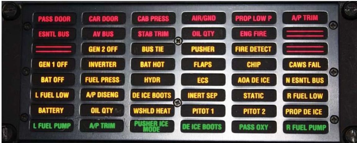
Figure 5. Central advisory and warning system display.
