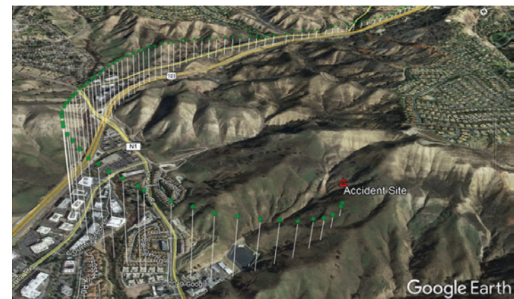
Figure 6. Radar tracking of last minute of the flightpath of the Sikorsky S-76B accident helicopter.
