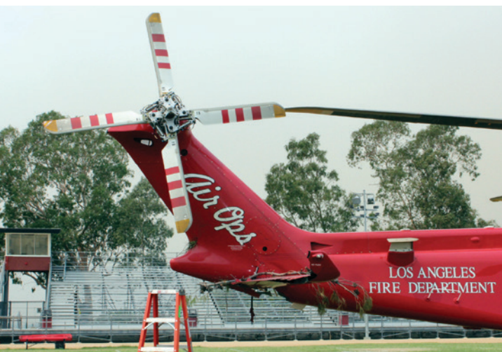
Figure 8. Damage to the helicopter's empennage, and embedded tree branches. SOURCE: LAFD
