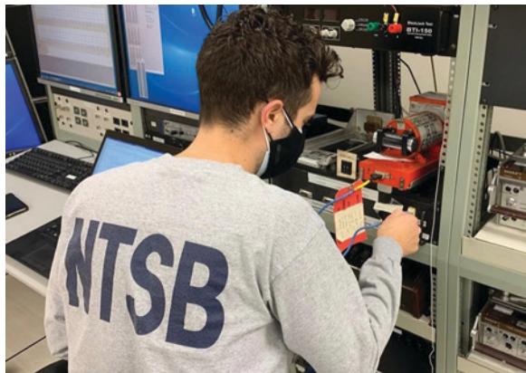
Figure 25. Vehicle Recorder Division staff member downloads the CVR from a United Airlines, Boeing 777 that experienced an engine failure shortly after takeoff from Denver International Airport on February 20, 2021.
