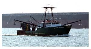
Figure 37. Langley Douglas with its outriggers extended and paravanes stowed at the end of the outriggers. PHOTO COURTESY OF STEVEN COLLINGWOOD
