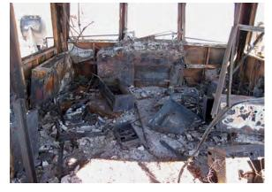
Figure 66. Charred remains of the wheelhouse.
