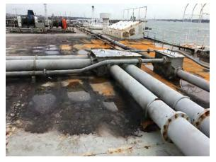
Figures 71 and 72. Above, damage to the top deck above the garage. Below, exterior bulkhead on the port side of the garage while looking aft.
