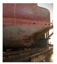
Figure 101. Damage to Nenita's bulbous bow, starboard side. PHOTO BY SPRING MARINE BULK, S.A. VESSEL GROUP FISHING
