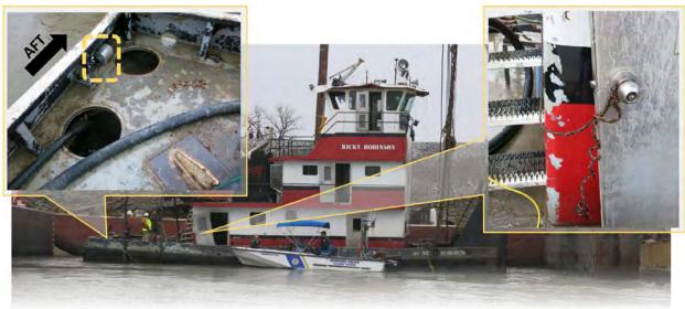
Figure 41. Ricky Robinson post-salvage. Two inset photos show (at left) both aft voids missing hatch covers, with a vellow square highlighting where the submersible pump was found, and (at right) the open starboard engine room door that was tied off to the stairs.
