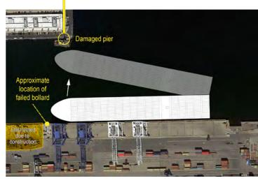
Figures 15 and 16. Above, damage to Black Falcon pier; below, approximate location and scale view of *Helsinki Bridge* alongside Conley Terminal and vessel's drift after breakaway. Also shown are area of terminal under construction and damaged pier at Black Falcon Terminal. (Satellite image shows a work barge engaged in repair of pier.) BACKGROUND FROM GOOGLE EARTH
