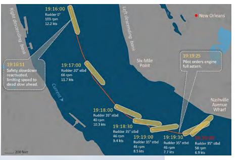
Figure 25. Trackline of the *Mia S* over the last 4 minutes leading up to the accident shows changes in the vessel's heading and speed over ground following an engine slowdown. BACKGROUND FROM GOOGLE MAPS
