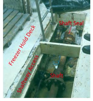
Figure 86. Shaftway of *Jake M*, a vessel with identical shafting to *Ben & Casey*, as viewed from the freezer hold while facing aft.
