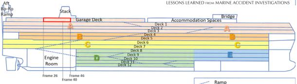
Figure 69. Simplified diagram of Honor's cargo decks and zones for CO<sub>2</sub> fixed firefighting system.
