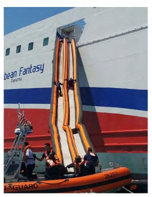
Figure 60. Caribbean Fantasy's marine evacuation system deployed on the starboard side. PHOTO BY COAST GUARD
