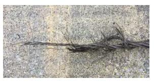
Figure 19. Strands on wire rigging that was recovered by investigators indicated that the wires had fractured while in tension.
