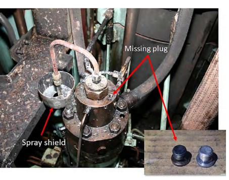
Figure 50. Fuel pump housing and top cover for the no. 6 cylinder, with missing pipe plug. The lower-right image shows the dislodged pipe plug (left) next to a new unused plug.
