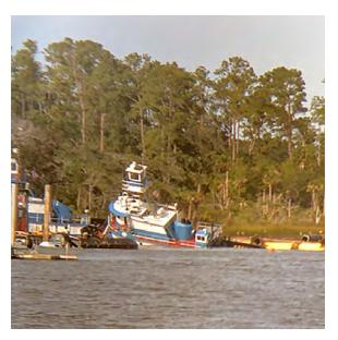
Figure 83. Atlantic Raider aground on the shallows of the west side of the Blount Island Channel. Note that the port quarter is under water up to the lower wheelhouse deck. PHOTO BY COAST GUARD
