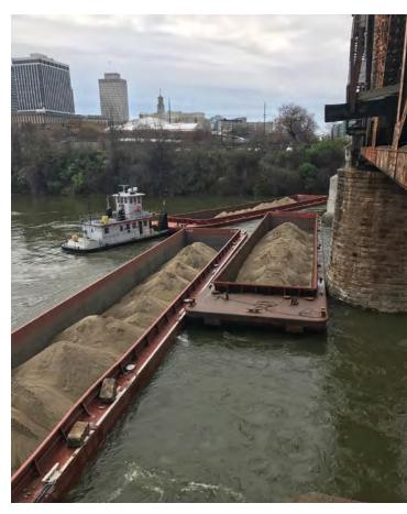
Figure 28. Barges from the *Steve Plummer* tow pinned against the upstream side of the CSX Railroad Bridge. PHOTO BY COAST GUARD
