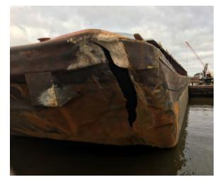
Figures 11 and 12. Damage from allision: (above) raked bow of port lead barge, *ART 35157*; (below) downstream view of the swing bridge's fixed pier near the left descending bank that was struck by the barge.
