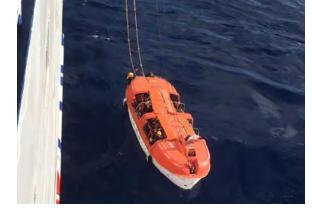
Figure 61. Lifeboat no. 1 in the water and unable to open the release hooks, about 0825. PHOTO BY A CARIBBEAN FANTASY PASSENGER
