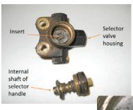
Figure 2. Fuel selector valve housing and section of selector handle (above) and fuel selector insert with fractured pieces (right).
