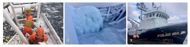
Ice accumulation on a vessel operating near the capsized vessel that was lost with all hands in the Bering Sea on February 11, 2017. (1, 2, and 3) *Polar Sea*: ice covers the decks and anchor chain during the vessel's transit to St. Paul Island on February 10 and remains on the wheelhouse while it was docked at the island the following day.
