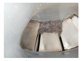
Figure 1. IGVs with material.
