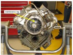
Figure 3. Compressor and bleed valve.
