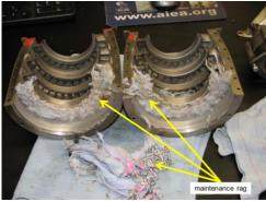
Figure 4. Compressor case halves removed.
