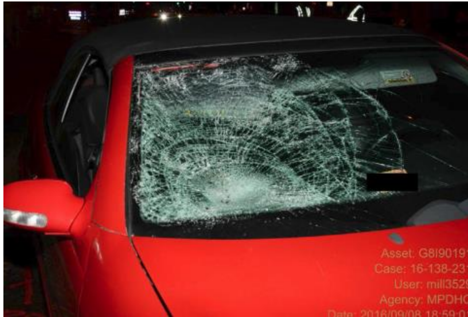
Figure 7. Damage to 2000 Mercedes-Benz sedan traveling straight on four-lane road at reported speed of 30 mph, Washington, DC, August 2016 (NTSB 2018m).
