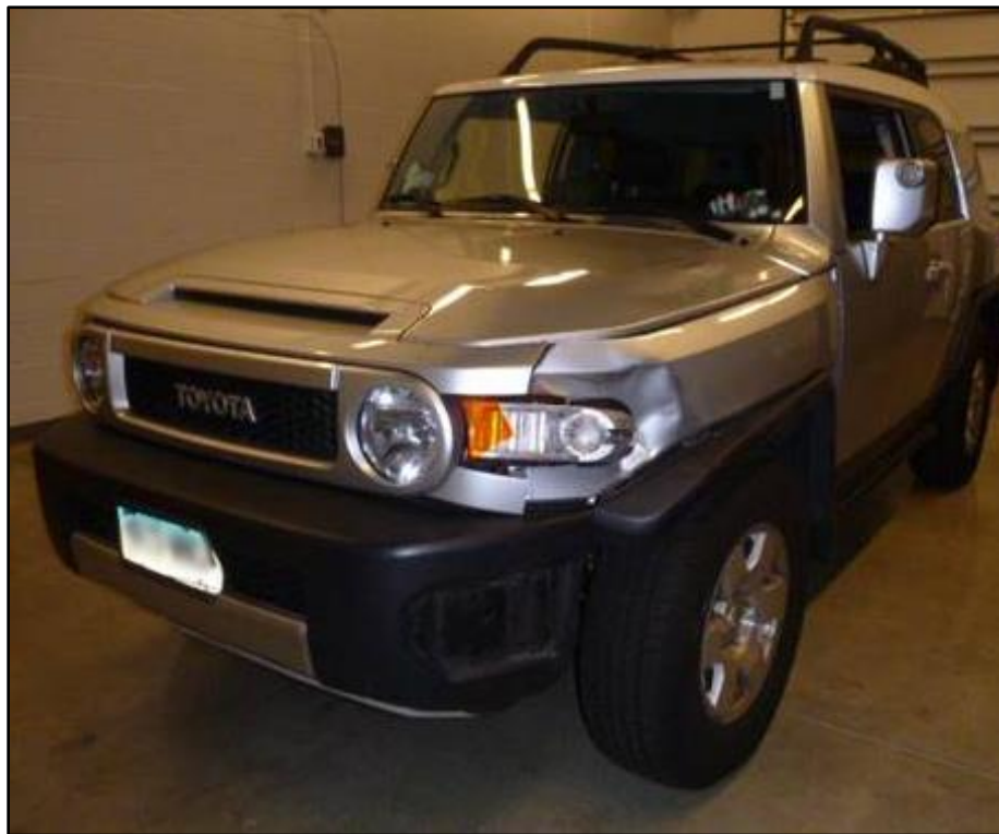
Figure 8. Damage to 2007 Toyota SUV traveling straight on two-lane road at reported speed of 30 mph, Old Saybrook, Connecticut, August 2016 (NTSB 2018l).
