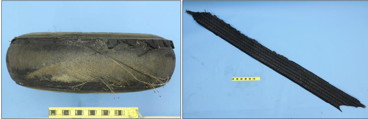
Figure 8. Carcass of left rear tire from the Lake City vehicle (left) and its delaminated tread (right).
